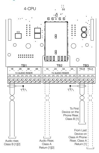
[1] For Class B risers, install a 15 k $\Omega$  EOLR at the last device on the riser. Do not install an end-of-line resistor if the riser is wired Class A.
